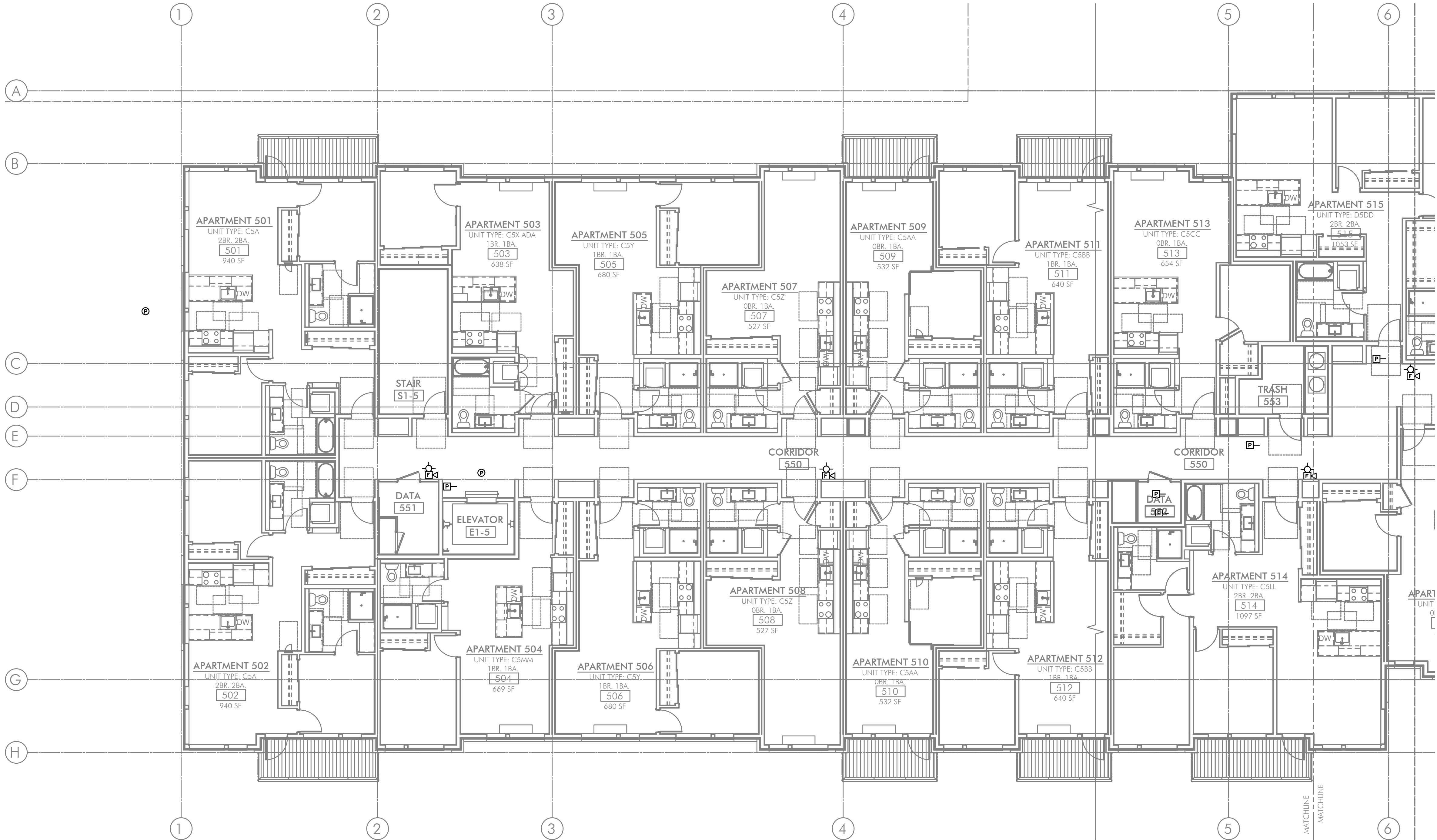
1 LEVEL 5 TECHNOLOGY FLOOR PLAN T3.05 SCALE: 1/8" = 1'-0"
