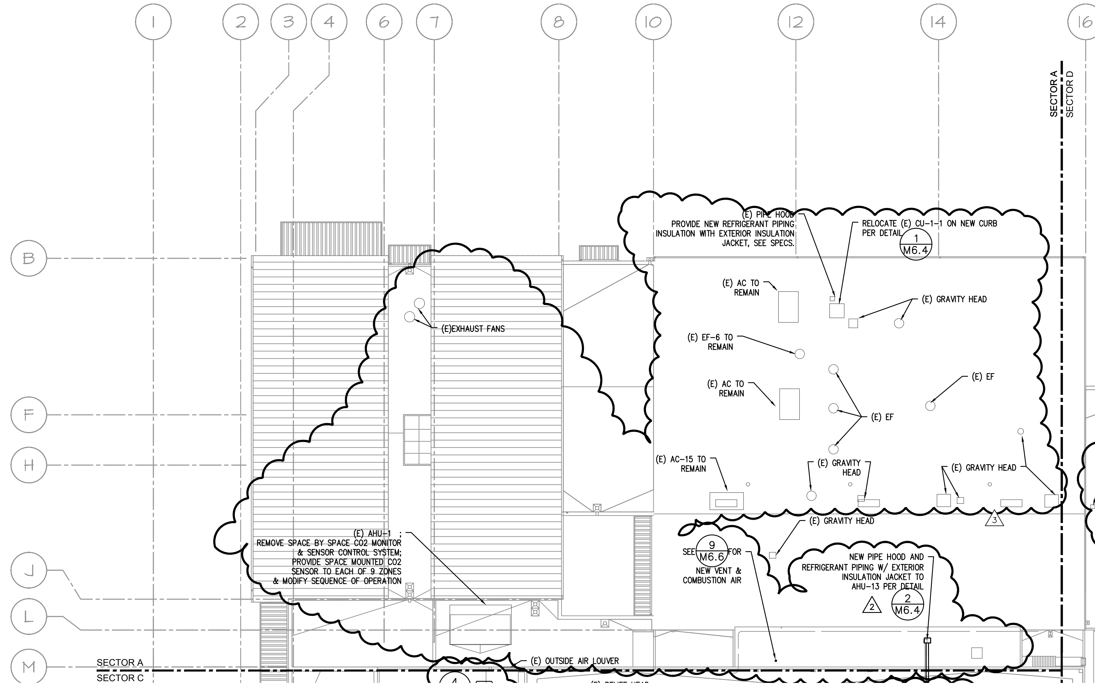
1 HVAC ROOF PLAN - SECTOR A M2.1 SCALE: 1/16"=1'-0"
