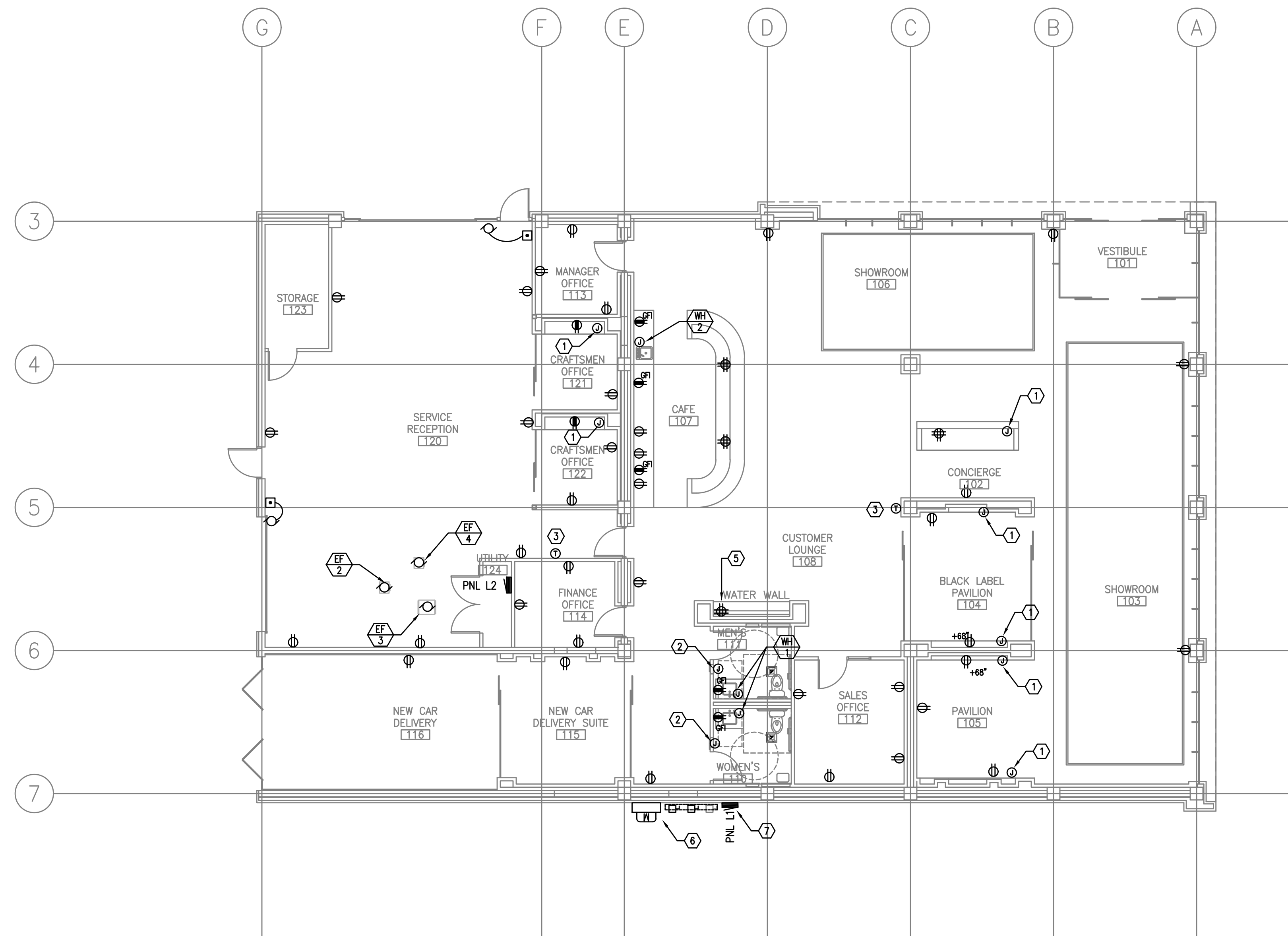
1 ELECTRICAL POWER PLAN E3.01 SCALE: 1/8" = 1'-0"
