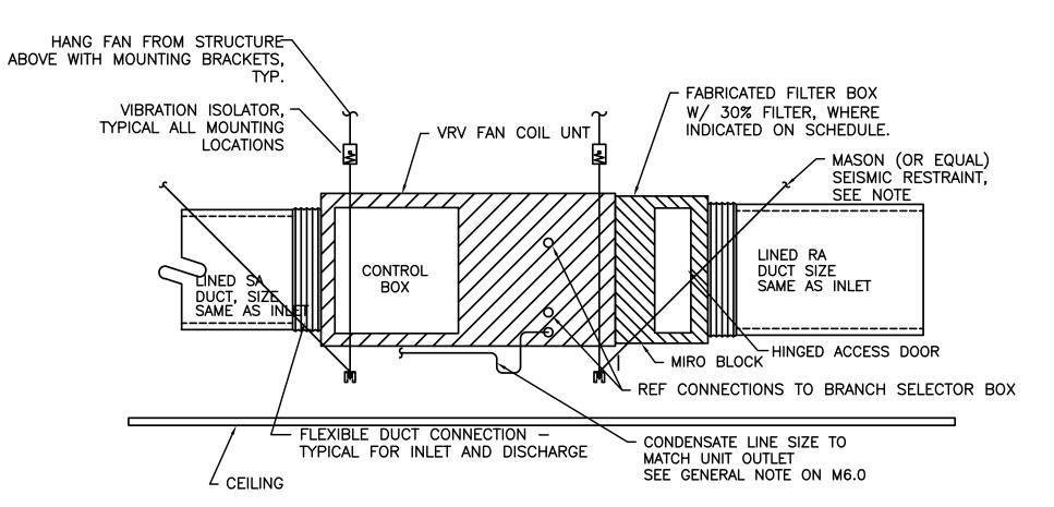
NOTE: LOCATE SUPPORT & SIESMIC TO MAINTAIN UNHINDERED ACCESS FOR MAINTENANCE OF UNIT.
