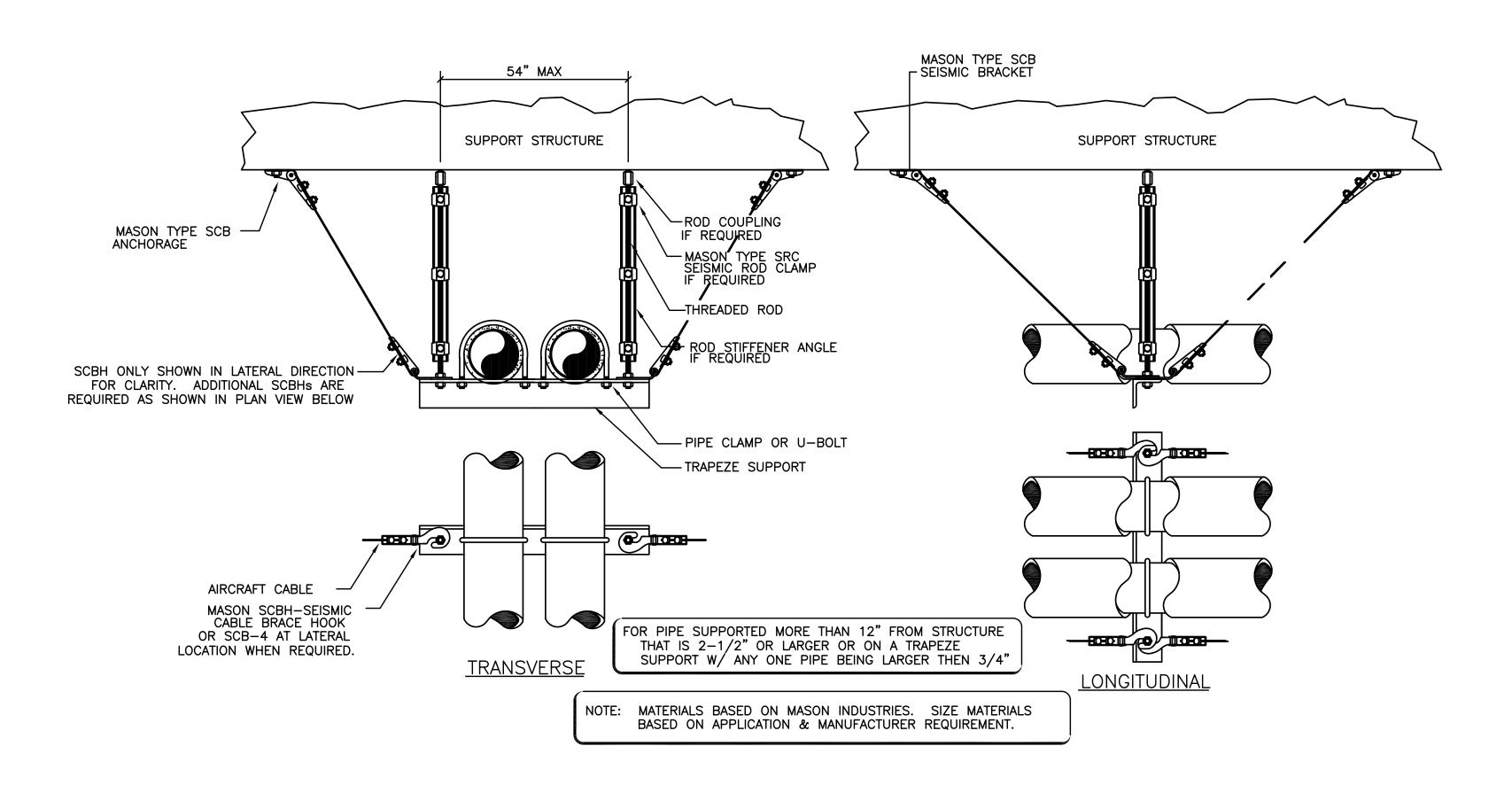
SEISMIC PIPE SUPPORT SCALE: DETAIL
