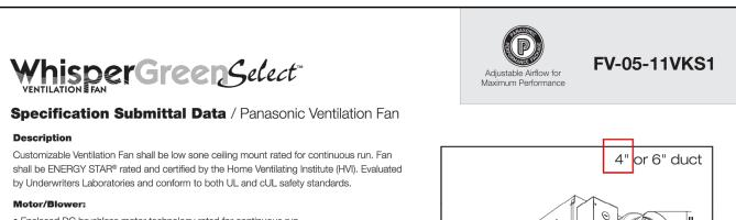
• Enclosed DC brushless motor technology rated for continuous run.
