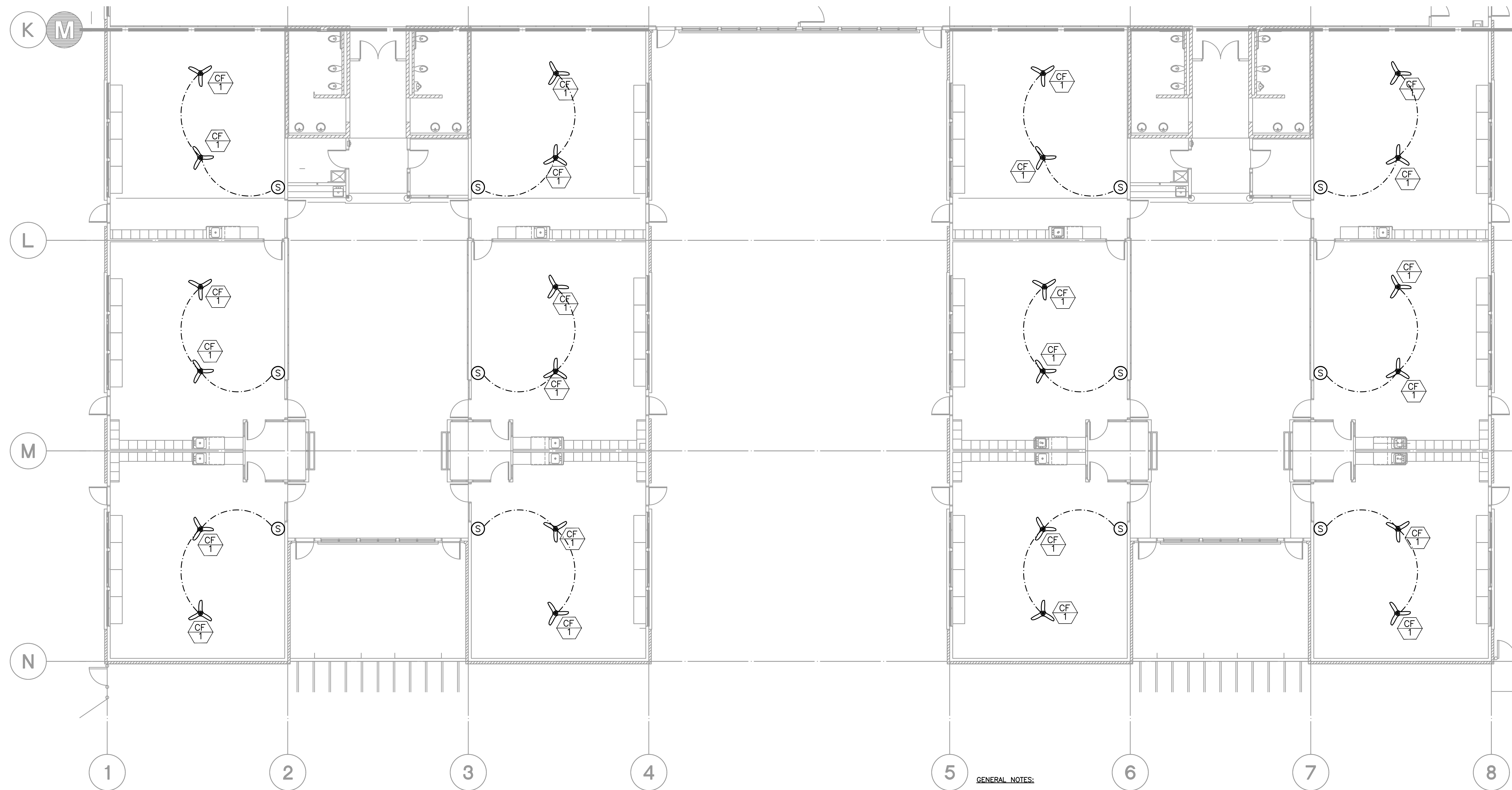
1 HVAC FLOOR PLAN— WING "C" AND "D" M1.4 SCALE: 1/8" = 1'-0"
