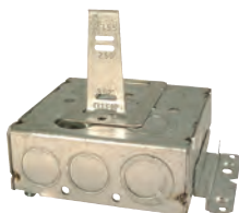
"UBS" Support Universal Back Side support to provide bracing on back of box for wall cavities 2-1/2" - 6" thick.
