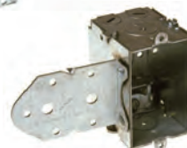
"LB" Bracket Face mounts on front edge of wood stud. Use when space between studs is limited. 5/8" offset to clear narrow door molding.
